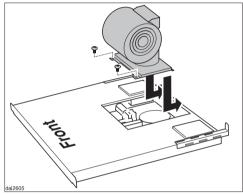
■ Mount the blower on the front of the ventilation system housing using the 2 screws while positioning the vent collar in the opening of the cover.
